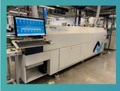
We have taken delivery of a second new reflow oven, widely regarded as the best in its class, with the 7 zone heat tunnel and a process length of over 4 metres. It offers the highest throughput, optimised energy balance, best process control and maximum machine up-times, with the "e" standing for efficiency.
