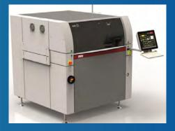
We have recently invested in another **DEK NEO Horizon screen printing** machine. With advances in machine design and technology, the new machine is far more accurate in the alignment of the stencil to the board. The coplanarity presentation of the board to the stencil is greatly increased across the board surface area giving a superior gasket seal between the board and stencil resulting in improvements in printing. The process repeat accuracy of the system is up to  $\pm/-20\mu m$ .
